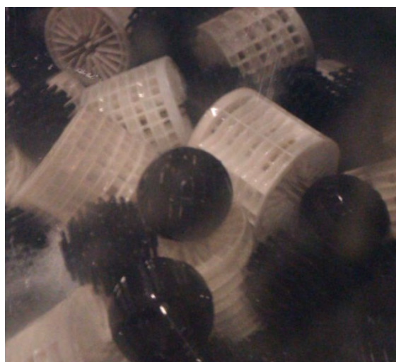
Figure 26 – Common biofilter media (large surface areas)
