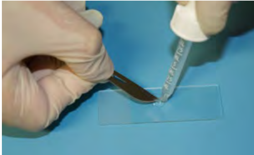
Figure 30 - Adding the water to the slide
